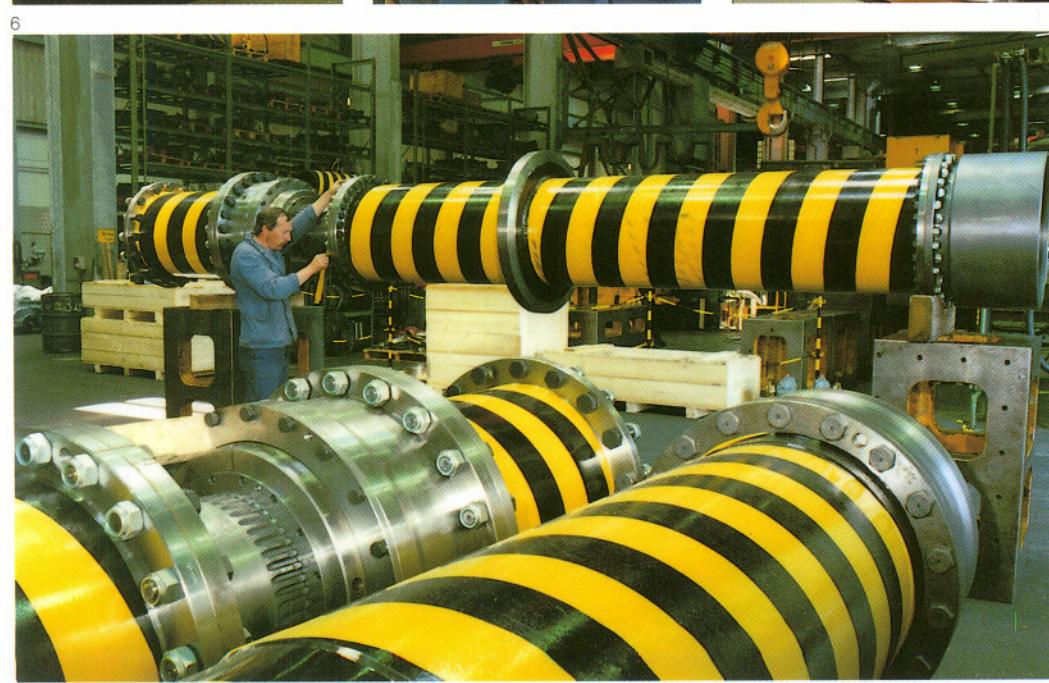
1 Vertical curved tooth couplings with brake disk for use in rudder propeller systems.
