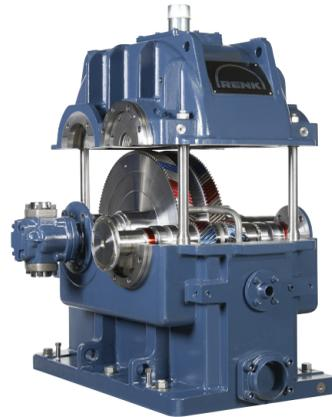
For the shaft bearings, plain journal bearings in an offset design are used that are optimized to perfection. For higher speeds, tilting pad journal bearings are installed. For bearing the gear shaft, one plain journal bearing is additionally provided with axial stop collars as a standard. Optionally, a separate axial thrust bearing can be installed.
